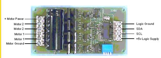
The Motor Ground and the Logic Ground are internally connected on the Module. Be sure to use cable rated for at least 5A for the Battery, Fuse and Motor leads.
